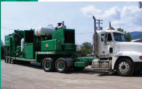
When abatement and profiling is required on larger projects, steel grit recycling minimizes waste management and disposal costs.
